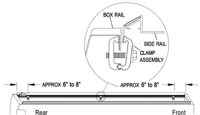
4. Place the tension control plate on the top of the side rail and place the pin in the first hole. This is the factory setting and will locate the T-Bolt in the front of the slotted hole in the side rail. Next, set the cover assembly behind the cab and feed the T-Bolt down through the tension plate and side rail. The header seal should be on the top of the bulkhead of the truck. **Use supplied flat, lock washer and nut and tighten front bulkhead assembly.**
