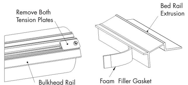
3. Place the front of the side rail and round gasket tight against the front of the truck box. Starting at the tailgate evenly space the 3 clamps along each side rail leaving approximately 6 to 8 inches on each end. To insure optimum performance and cover fit, the **side rails must be level**. To adjust the rails, loosen the screws and reposition the clamp higher or lower on the truck bed rail lip. **Make sure to tighten all clamps!**
